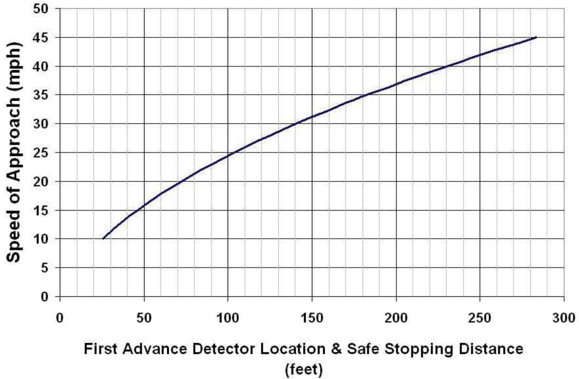
Figure 4-20 Detector location for multiple detector technique (level approach)
